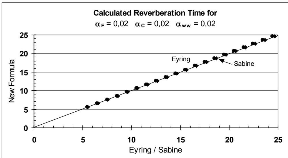
Figure 1. Calculated reverberation time for little absorption of all surfaces.
