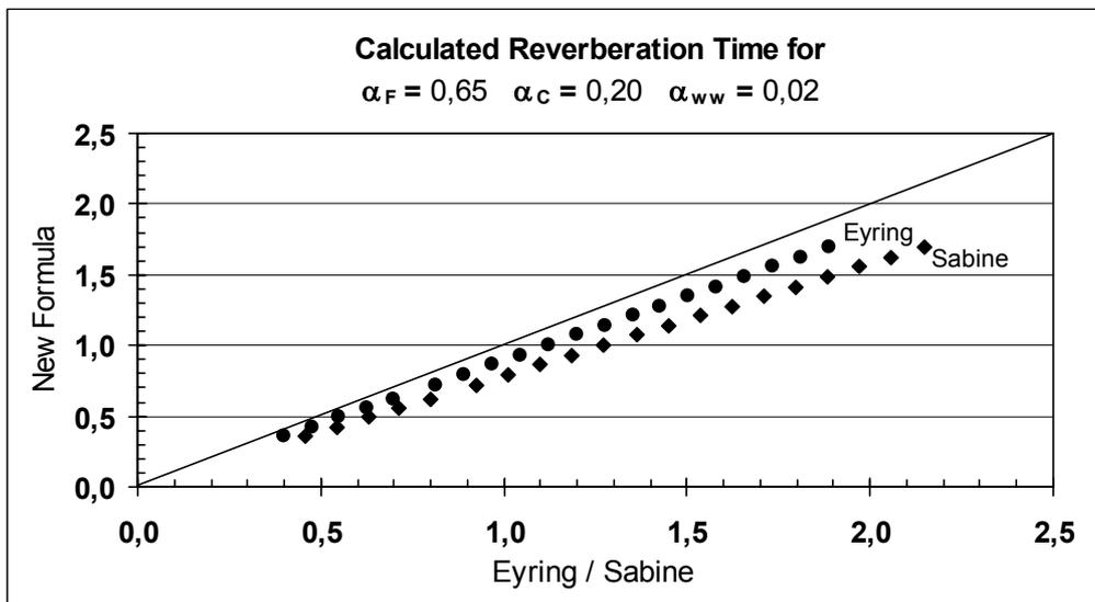
Figure 3. Calculated reverberation time for non-uniformly distributed sound absorption.
