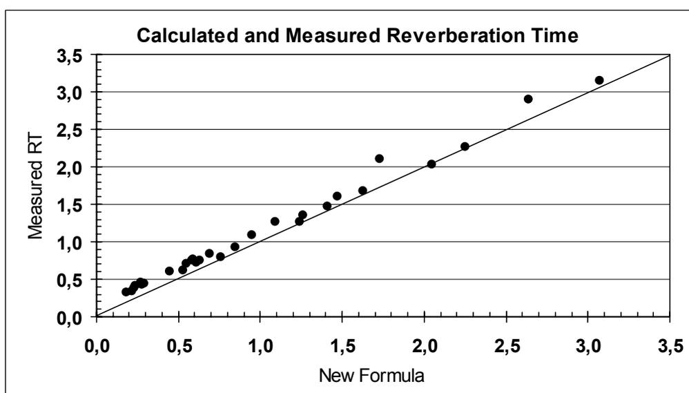
Figure 4. Measured and calculated reverberation time with “fitted” absorption coefficient.
