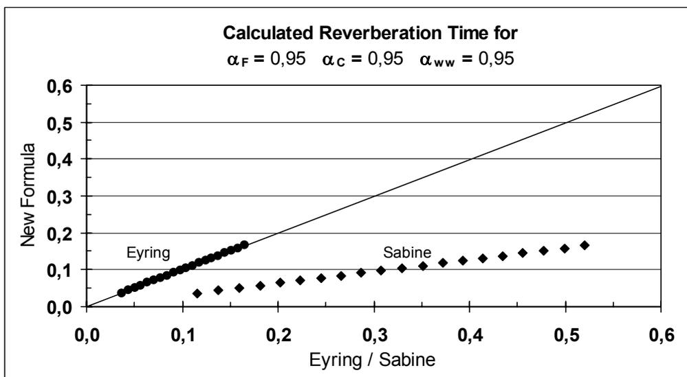
Figure 2. Calculated reverberation time for high absorption of all surfaces.
